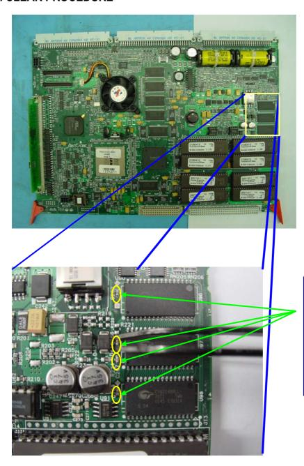
To crash the Mk6 main board these capacitors need to be shorted C269, C267, C266 & C262 Use a pair of tweezers to short the capacitors
